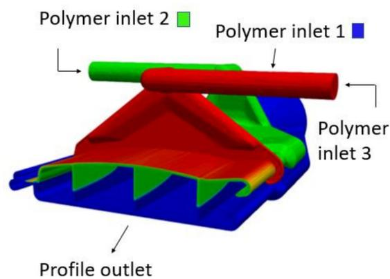
Figure 1 – Pool cover co-extrusion die setup
