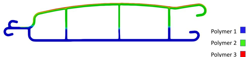
Figure 4 – Pool cover cross sectional area
