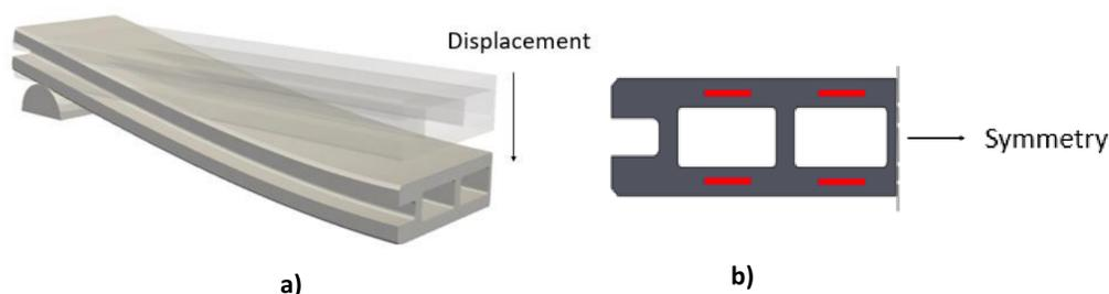
Figure 2 – Pool deck profile flexural simulation setup a) and its cross sectional area b)
