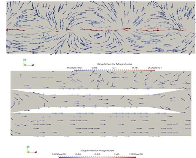
Figure 3: Vector plots showing (a) orbital flows in absence of pipe and (b) reversible flows inside the pipe. Time period of wave, T=1.0 second and wave height, H=0.02 m
