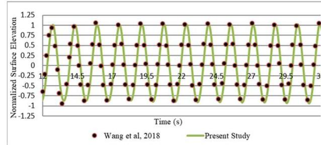
Figure 1: Normalized surface elevation history at 3 m downstream of the piston location
