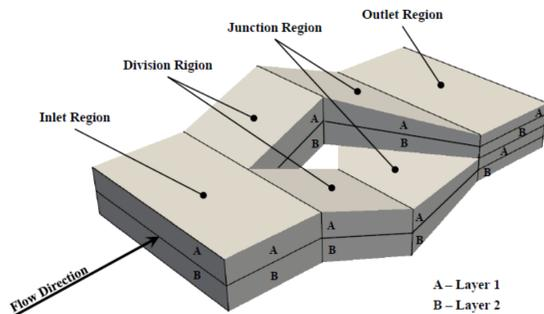
Figure 1. Interfacial surface generator module.
