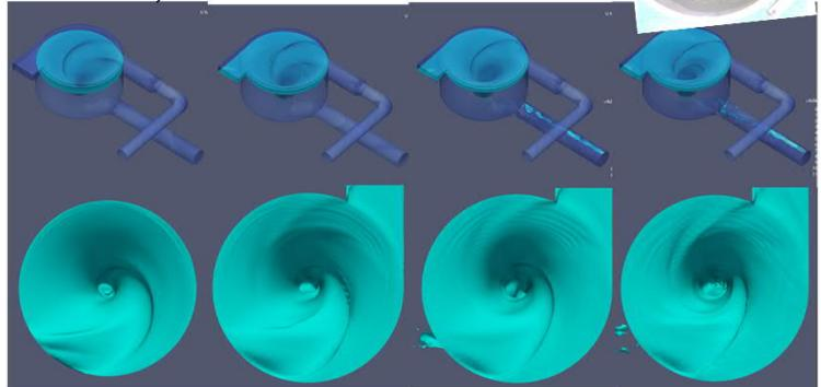
Fig.3 Water surface predicted with various turbulence models
