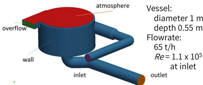
Fig.2 Simulation model
