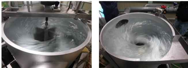
Fig.1 Low Rotation Tub-Type Water Wheel with and without blade
