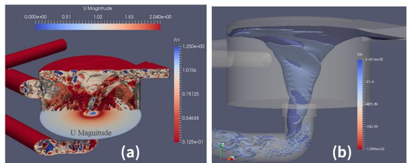
Fig.4 Strong depression regions: (a) RC correction term is effective in red region where rotating velocity is large. (b) A steep density gradient around water surface depresses turbulence with the effect of the buoyancy term.
